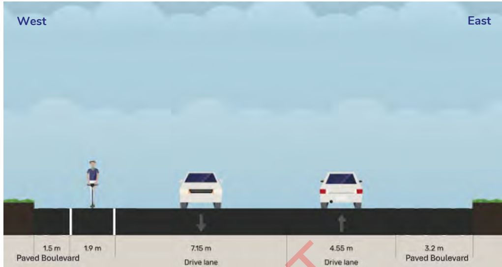
Figure 11: Existing Northern 4th Street Cross-Section Between B Avenue and A Avenue
