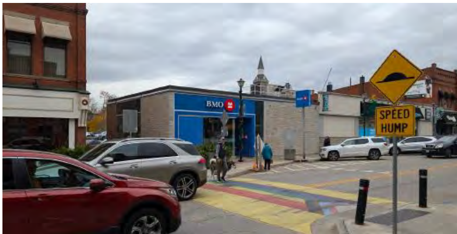
Figure 5: Example of raised mid-block crosswalk
