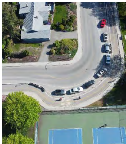
Example of a road in Kelowna, BC after being narrowed with bi-directional bike lanes.
