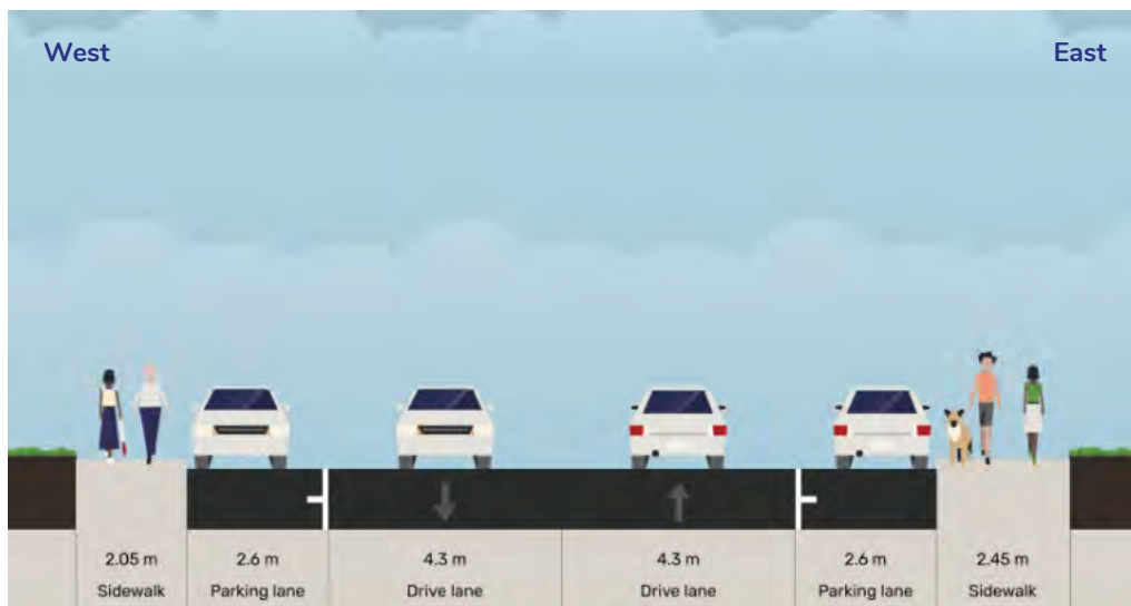
Figure 11: Existing 4 th Street Cross-Section Between A Avenue and Front Street
