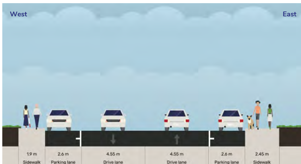
Figure 13: Existing Southern 4 th Street Cross-Section Between B Avenue and A Avenue
